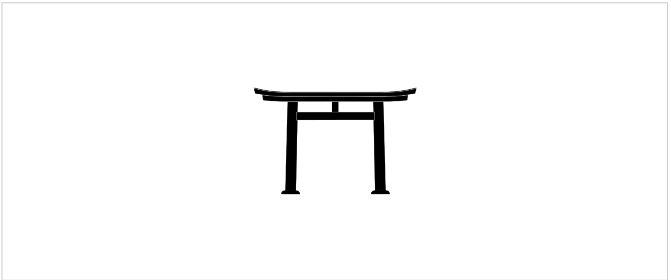
Nakayama torii – a myōjin torii , but the nuki does not protrude from the pillars.
