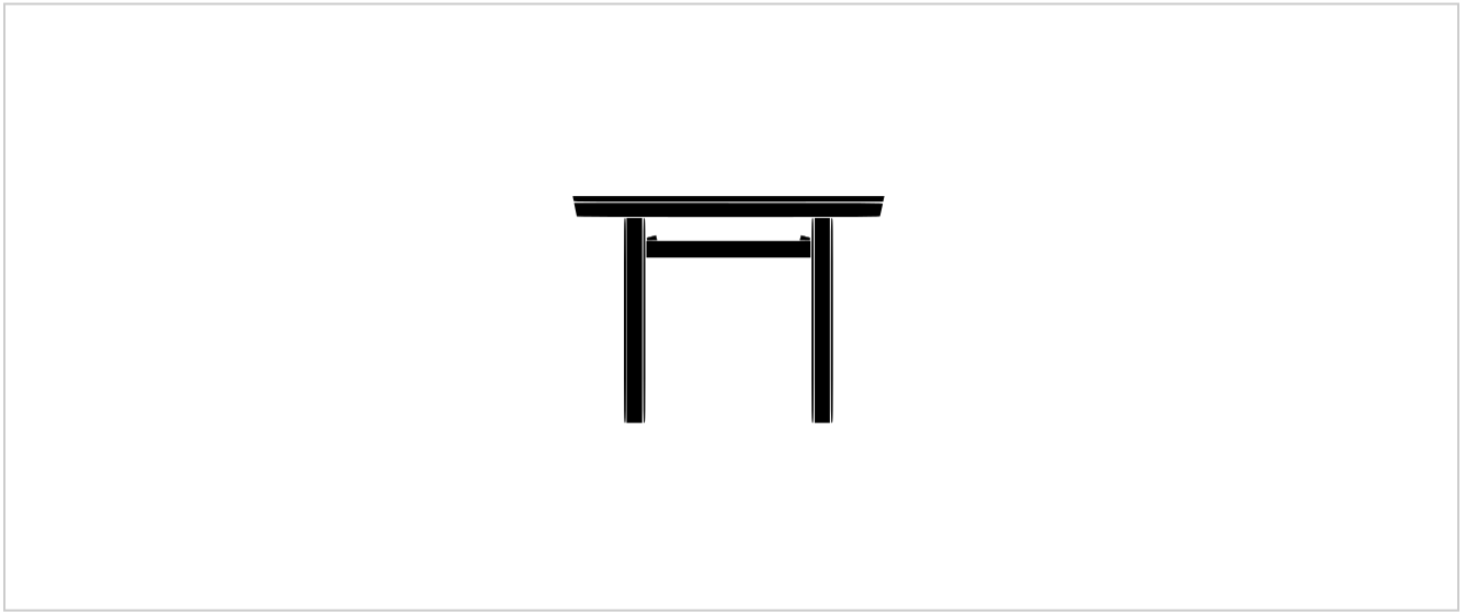
Ise torii – a shinmei torii with a kasagi pentagonal in section, a shimaki and kusabi.
